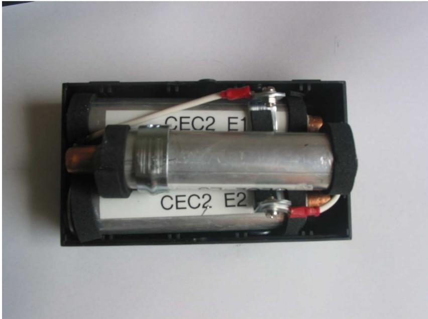
This type of converter consists of 3 crystal elements in series connection that produce enough energy for a LED.
