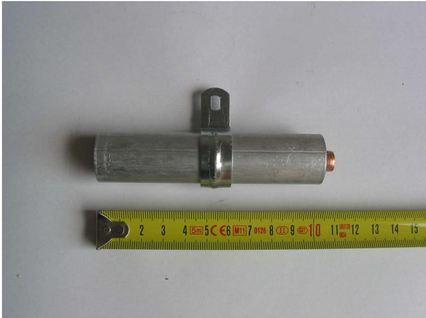
Each crystal element consists of an outer aluminum and an inner copper tube which serve as electrodes.
